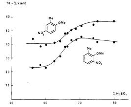
Figure 3. Nitration of o-methoxytoluene.
